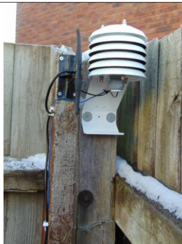
External mounting of radiation shield and 4G network antenna.
