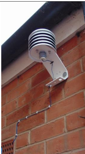
External mounting of radiation shield.
